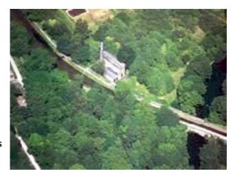
The structure is 182.9 metres long, 9.1 metres high and supported by three arches. The one which spans the river is nearly 73 metres in length. There are two date stones above this central arch.
