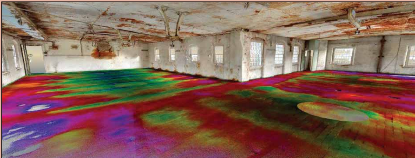
DATA DISCOVERY: Scanning in Darley Abbey Mills, with the floor coloured by elevation, revealed the worn paths made by mill-workers as they serviced the machines, shown here in red.
