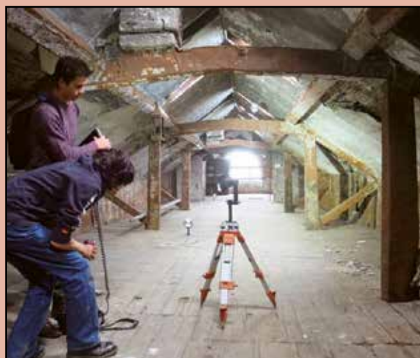
DATA DISCOVERY: Scanning in Darley Abbey Mills, with the floor coloured by elevation, revealed the worn paths made by mill-workers as they serviced the machines, shown here in red.
