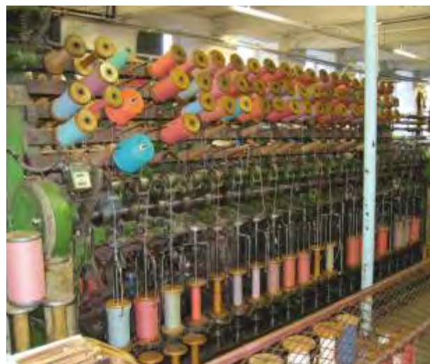
Fig.5.12 Cotton doubling machine, installed at Masson Mills following manufacture in 1954 by Prince-Smith and Sells Ltd of Keighley, West Yorkshire. The doubling frame combines the process of drawing the cotton yarn with twisting of the yarn to give it strength ( www.massonmills.co.uk/Museum/M/ ); reproduced by courtesy of Robert Aram)
