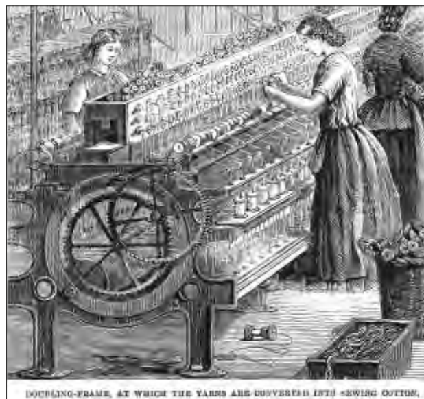
Fig. 4.38 Boar's Head Mills, Darley Abbey: working the doubling-frame machines (Illustrated Times, July 1862; image courtesy of Derbyshire Local Studies Libraries and www.picturethepast.org.uk : DRBY004963)
